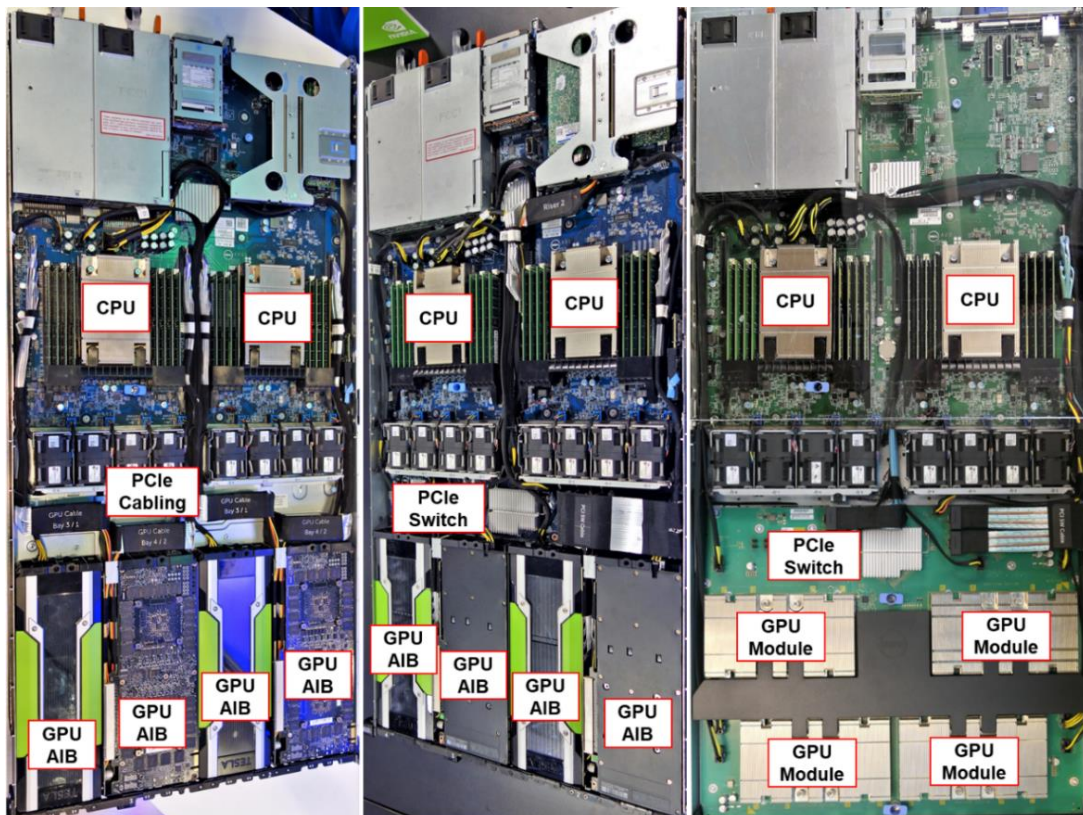
Figure 3: PowerEdge C4130 / C4140 CPU to GPU Connection Options
